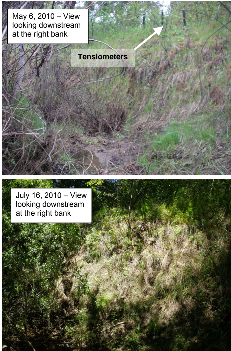
Figure 12. Photos taken of the bank stability study site on the Southwest Tributary before and after the high-flow releases. Note the absence of bank failure and the increase in herbaceous vegetation coverage on the bank surface.
